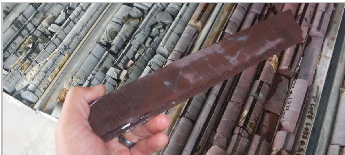
Figure 23.5 Anglo drillhole BKS3 (just north of the Bullion Kraaipan Project area) iron rich sediment and BIF (source: Author).
